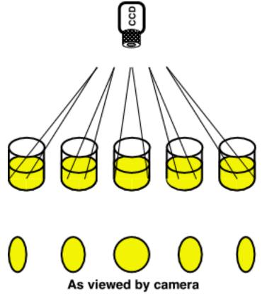
Raising the camera will mitigate the situation somewhat at the expense of a lower overall intensity at the detector. Geometric weighting patterns can be applied to correct for the edge intensity loss, however, the signal to noise ratio for the outer wells must be worse than for the central wells.
